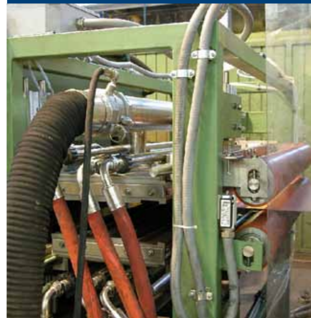
Metal strap-de-greasing system Belt width: up to 2 m
